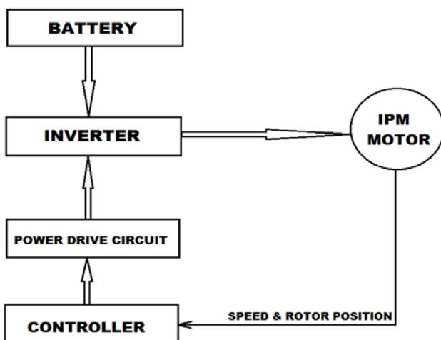
Fig.1 Block diagram showing Electric Propulsion System in Electric Vehicle
